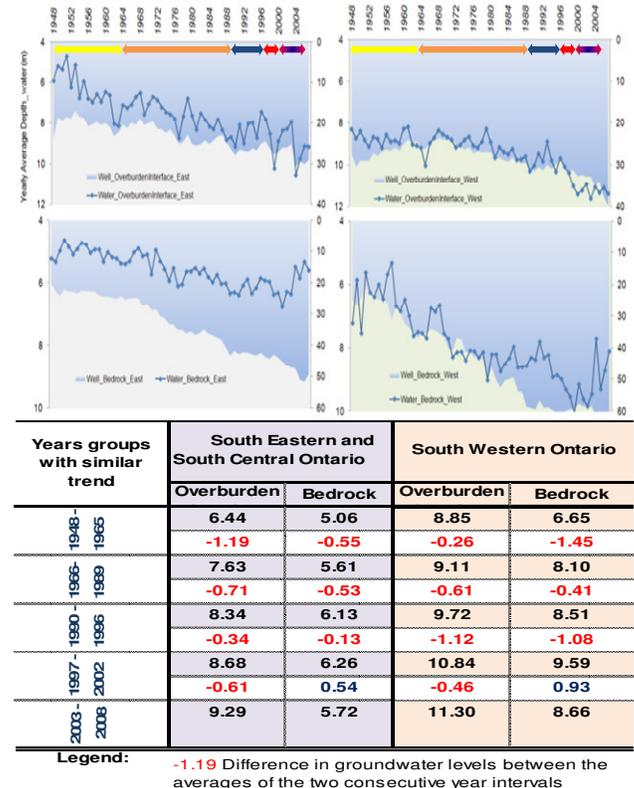
Figure 3. Mean yearly depth to water and well depth variations for the different aquifers and for the different areas (upper figure) and breakdown of the variation (table)
